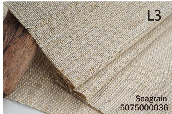
Weight:446gsm Width: 244cm | 96inches Material: JUTE 100%
